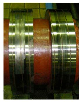
install the rounding brushes weekly. After nearly a year of operation in this manner, an unplanned outage occurred and inspection revealed that some locations of the rings, had up to 0.090 inches of metal removed. The plant was never able to get support from the contractor or independent representative at solving the ongoing arcing and photographing problems and contacted Cutsforth for a long-term solution.
