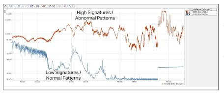
**A Tale of 2 Generators:** The Red Line Generator has Isophase Bus issues (specifically relay actuation); the Grey Line Generator is normal. With EMI, plants can track generators side by side as another method to determine when a fault is occuring, and take appropriate action.
